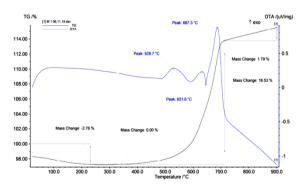
Fig. 1. TG-DTA curve of milled sample with 11.2 mm balls, 2 h milling, sintered at 630  $^{\circ}$ C at 2 h with argon flow rate of 10 cm<sup>3</sup>/min
