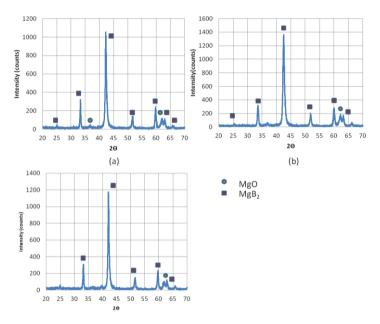
Fig. 2. XRD patterns of samples sintered with different argon flow rates, (a) 1, (b) 3 and (c) 5 cm<sup>3</sup>/min
