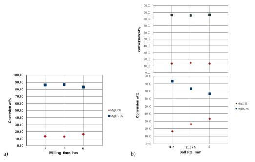
Fig. 4. MgB<sub>2</sub> phase wt % variation of samples according to different treatment times; 2, 4 and 6 h (a) and different size of balls for 2 and 6 h, respectively (b)
