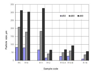
Fig. 6. Particle size measurement results of samples milled at BPR of 6:1 with toluene as a process control agent
