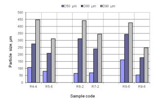
Fig. 5. Particle size distributions of samples milled with different ball sizes
